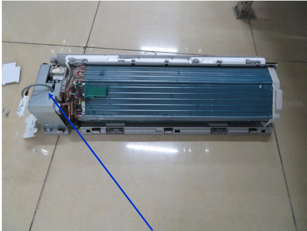
Main power box
